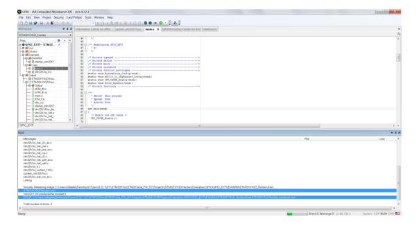
Mastering the application means that the IDE/C-Trust encrypts and signs the embedded application package to be accepted by the SBM (secure boot manager).
